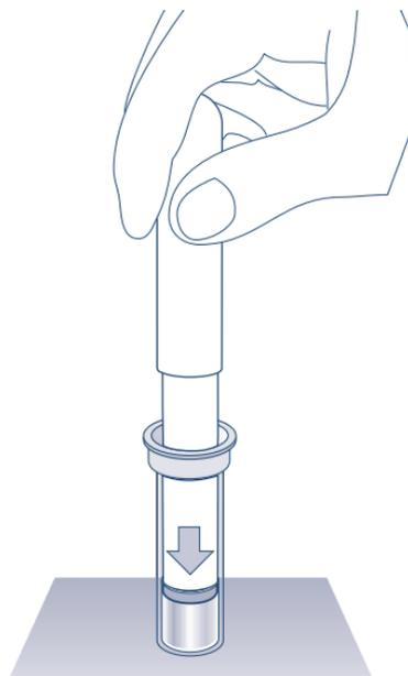
*Push the plug **FULLY** into the tapered end of the spin column using the plug insertion tool.*
