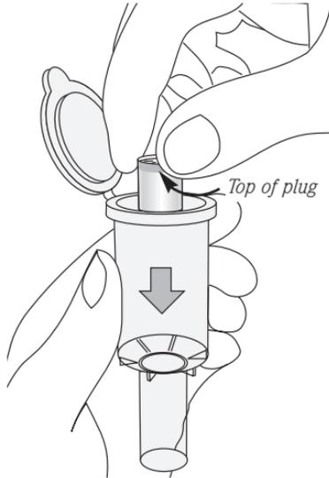
*Place the plug into the spin column with the recessed tapered end uppermost.*
