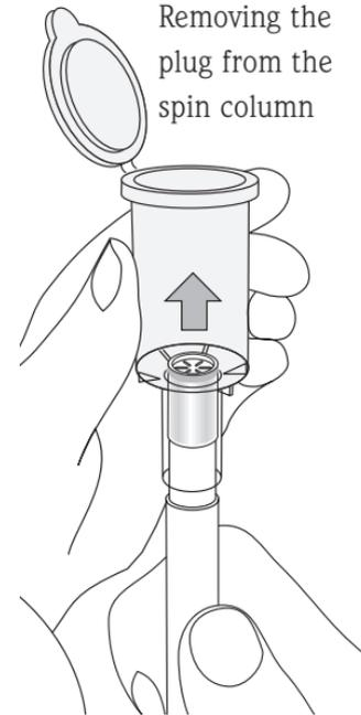
Removing the plug from the spin column
