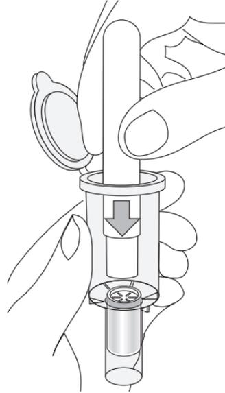
*Push the plug **FULLY** into the spin column using the plug insertion tool.*
