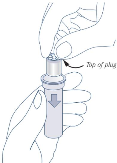
*Place the plug into the spin column with the recessed end uppermost.*
